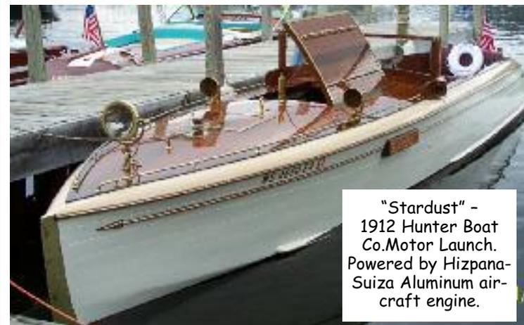
"Stardust" - 1912 Hunter Boat Co. Motor Launch. Powered by Hispana-Suiza Aluminum aircraft engine.
